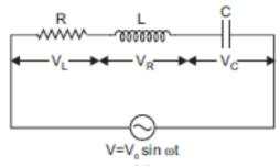
Since L, C and R are connected in series, current flowing through them is the same. The voltage across R is  $V_R$ , inductance across L is  $V_L$  and across capacitance is  $V_C$ .
