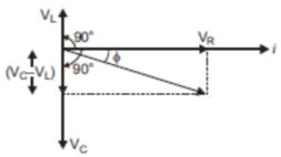
Thus,  $V_R$  and  $(V_C - V_L)$  are mutually perpendicular and the phase difference between them is  $90^{\circ}$ . As seen in the fig, we can say that, as the applied voltage across the circuit is V, the resultant of  $V_R$  and  $V_C$  -  $V_L$ ) will also be V.
